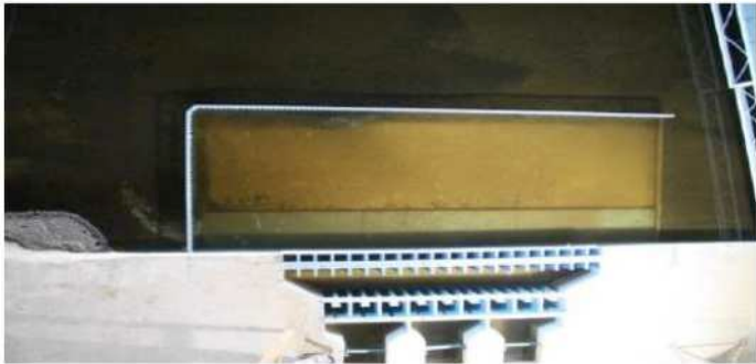
Fig. 9 Sedimentation inside the basin after introducing the deflectors after long term operation (Sediments in black)
