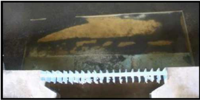
Fig. 5 Deposition progress in the vicinity of the intake. Sediments are shown in black (baseline case before the deflectors)
