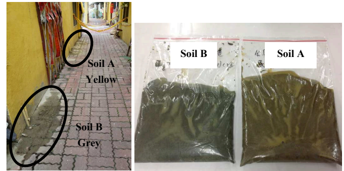
Fig. 6 Different colored sand boil samples
