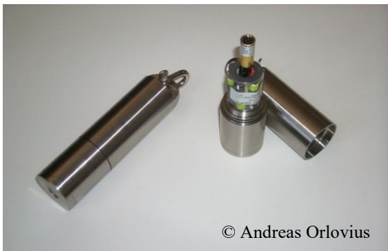
Figure 2: Absolute pressure probes, Driesen + Kern GmbH, type P-LOG125-B and P-LOG520-A (left) and post-processing of field observations (right).
