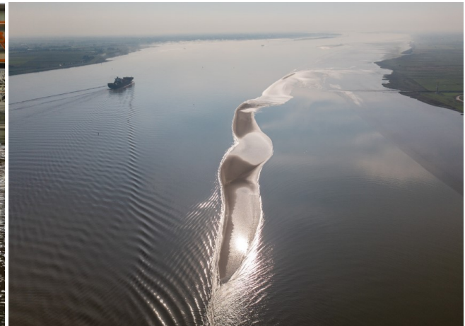
Figure 5: The secondary wave field of a container-ship deformed in vicinity to a sand bank due to shallow-water processes (Source: German Federal Waterways Engineering and Research Institute).
