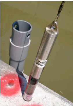
Fig. 7 Pressure-type sensor for flooding depth measurement
