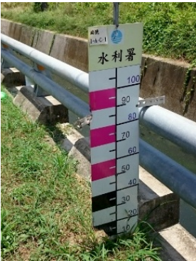
Fig. 6 Staff gauge for flooding depth measurement
