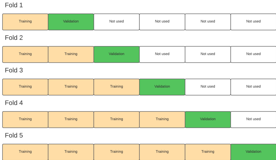
Figure 9, 5-Fold Walk Forward validation
