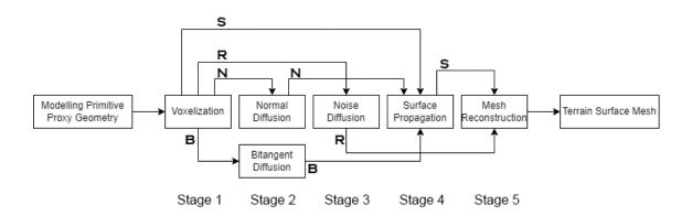
Figure 2.4: GPU computational pipeline for 3D sketching method proposed by Becher et al. [28]
