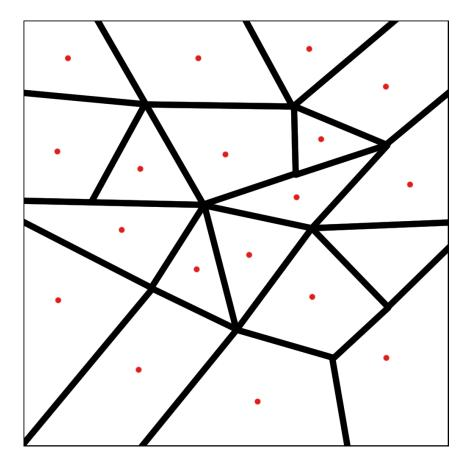
Figure 2.3: An example of a Voronoi cell diagram. Cells begin to expand from the red dots, partitioning the plane into their respective areas which are bound to their cells.
