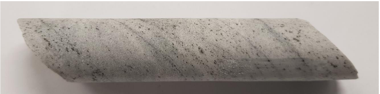
Figure 18. A piece of the drill core MM-196 taken from the depth of 73 metres. Sericite quartz sequence shows schistosity. Photo: Geological Survey of Finland.
