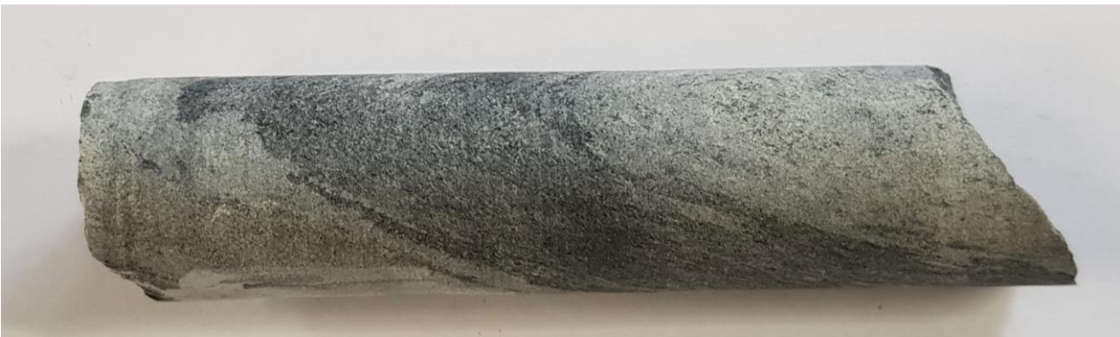
Figure 17. A piece of the drill core MM-190 taken from the depth of 105 metres. The amphibolite sequence dominates the beginning of the drill core. Photo: Geological Survey of Finland.
