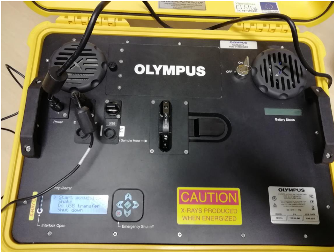
Figure 22. The front panel of Olympus Portable Onsite X-Ray Diffraction (XRD) Terra-542 device. Photo: Jenniina Siira.
