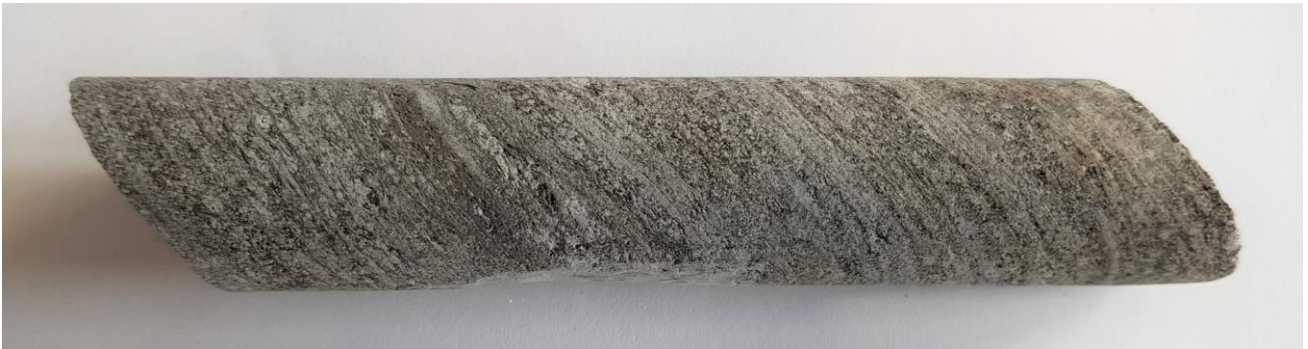
Figure 19. A piece of the drill core MM-198 taken from the depth of 43 metres. Dark sulphidic mineral grains are visible in the amphibolite (hornblende gneiss). Photo: Geological Survey of Finland.
