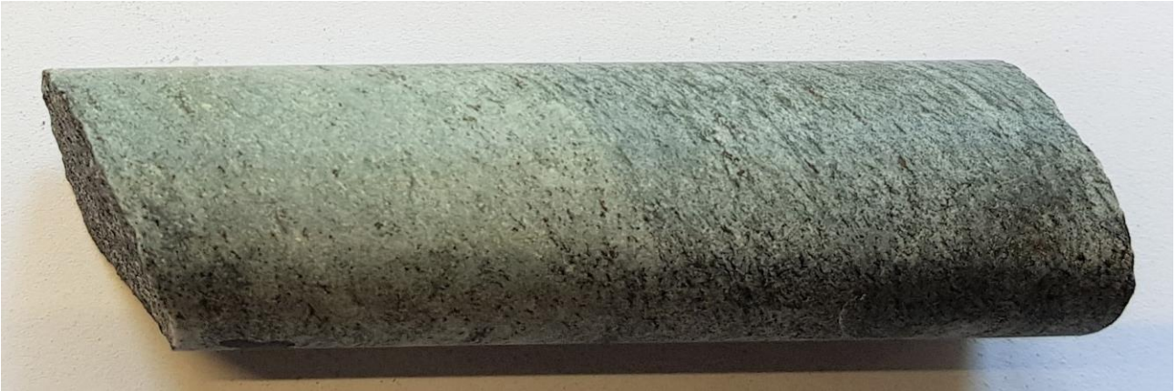
Figure 21. A piece of the drill core MM-241 taken from the depth of 125 metres from the amphibolite sequence. Photo: Geological Survey of Finland.
