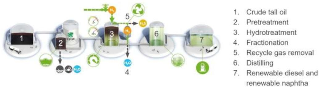
Figure 1. CTO-based renewable fuel production process.
