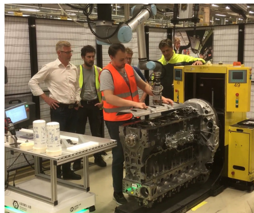
Figure 9. Collaborative robot assembly station controlled by a network of ROS nodes. Video clip showing the demonstrator: https://youtu.be/TK1Mb38xiQ8 , accessed on 24 May 2022.
