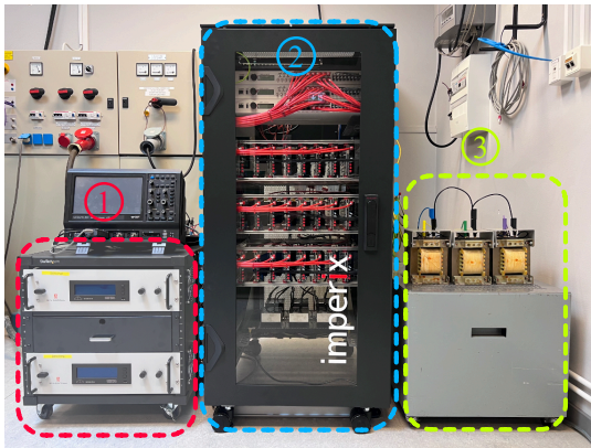
Figure 5.9: Lab set-up of the MMC: 1) DC power supply 2) MMC 3) Three-phase RL load
