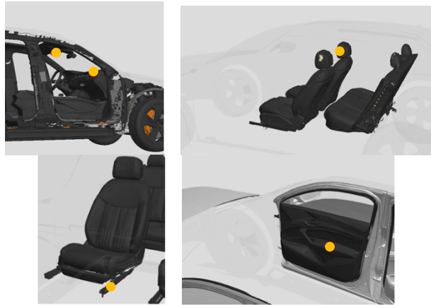
Figure 2. The location of the installed cameras (upper left), microphone (upper right), seat rail accelerometer (lower left) and armrest accelerometer (lower middle).
