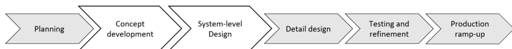
Figure 2.1: The generic process to engineering products and systems adapted from (Ulrich et al., 2020).
