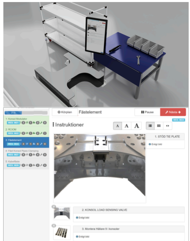
Fig. 4. Concept for the digitalized presentation of information at case B: workstation (top) and a screenshot of an example for experienced operators (bottom) (Asklund & Eriksson, 2018).
