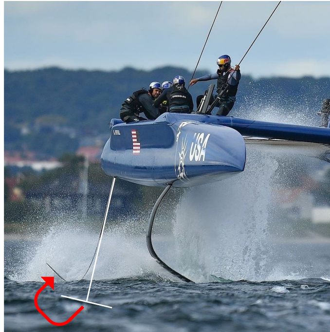
Figure 2. Example of large rudder deflection during sailing load of the Team USA high-performance catamaran from the F50 fleet in a SailGP event.
