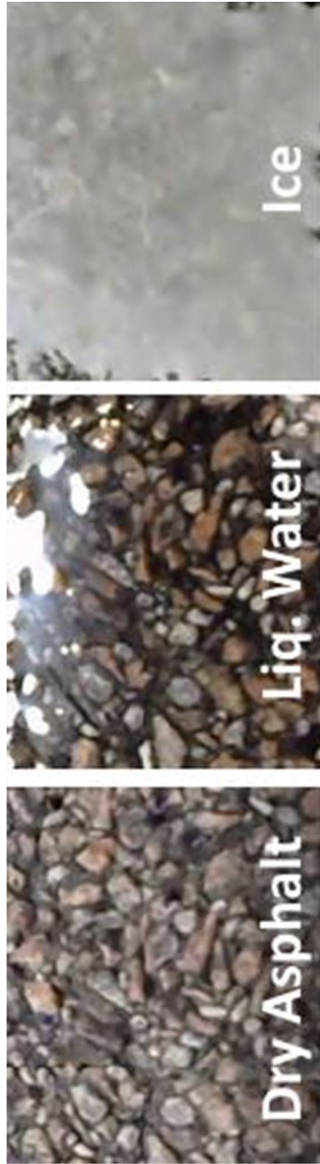
Fig. 6 Surface conditions studied in a laboratory-controlled environment. From left to right are dry, water, ice on the asphalt surface
