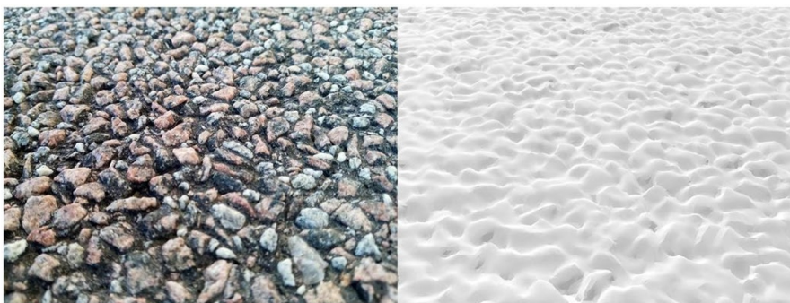
Fig. 3 Asphalt road surface used in the study (left) and its 3D scan (right)
