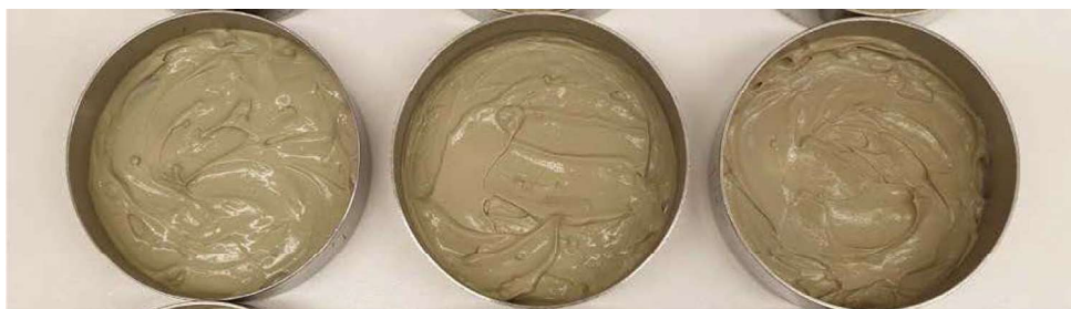
FIGURE 7 Fresh precipitate from LS4 in which the alkali extraction time was 1 h (left), 2 h (middle), and 3 h (right)
