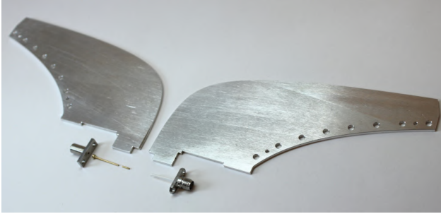
Figure 3.3: Coaxial single-ended excitation feed-through for a ridge-pair.
