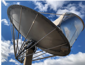
Figure 1.6: Reflector in the Allen Telescope Array (ATA) with shroud shielding against ground. Image credit: Alex Pollak, ATA/SETI.
