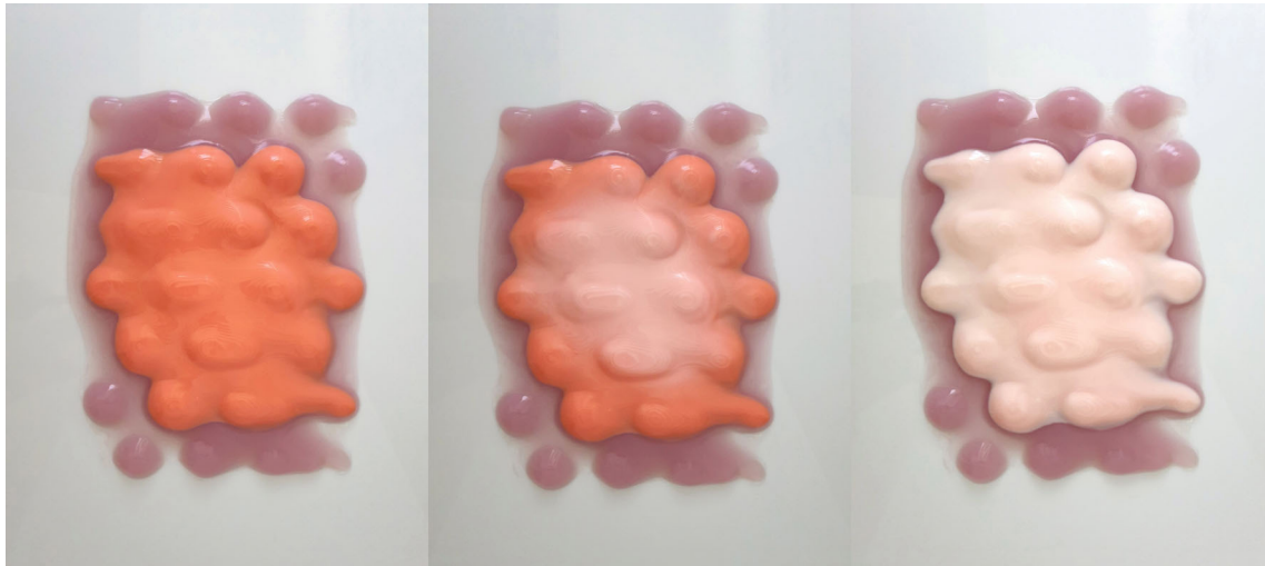
FIGURE 22 A surface design strategy based on animate reshaping, achieved with thermochromic pigments. The model seen in daylight, with gradual color transition induced by gradual surface temperature change
