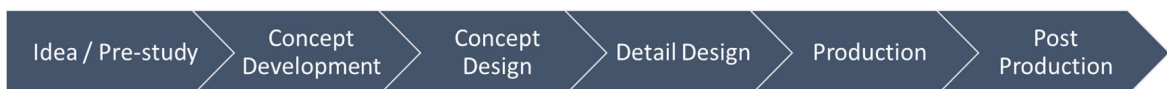
Figure 2. Generic phases in the project development process. The entry point of the design–build contractor can vary depending on when the procurement of the design–build contractor occurs but should, at the latest, be in the ‘detail design’ phase.
