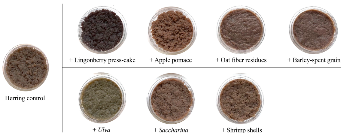
Fig. 3. Appearance of protein isolates produced from herring co-products in the absence and presence of helpers by the alkaline version of pH-shift process.
