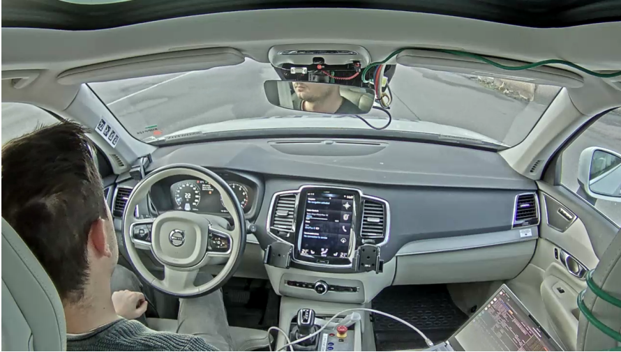
Figure 4.4: The vehicle is being controlled by solving an OCP on a laptop computer, and sending the actuation requests through a network connection through OpenDLV.
