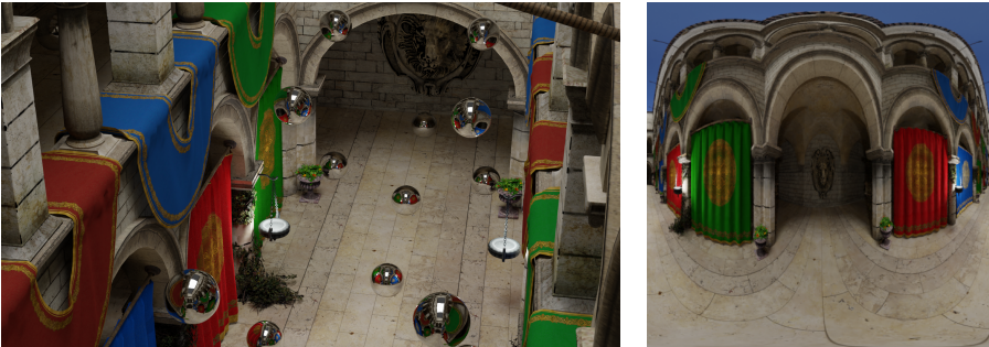
Figure 1.4: Left : A scene with a few reflection probes, displayed as spheres (only visible when building the scene, not during normal rendering of the scene). Right : What the map rendered for one of the reflection probes would look like.
