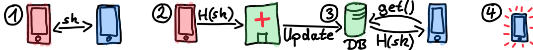
Figure 2. The parties use their shared secret ( sk ) to anonymously notify each other using the health authorities’ public database. When in contact, devices exchange a secret key (1). Upon infection, the infected party collects the relevant anonymous notifications, which the health authorities publish in their database (2). All users download the data and check for matches on their devices (3). The devices report matches back to the user (4).
