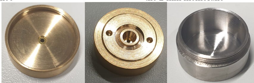
Figure 6.2.5 Photos of the Knudsen cell. From left to right: bottom view of the brass lid, top view of the brass lid, steel container.
