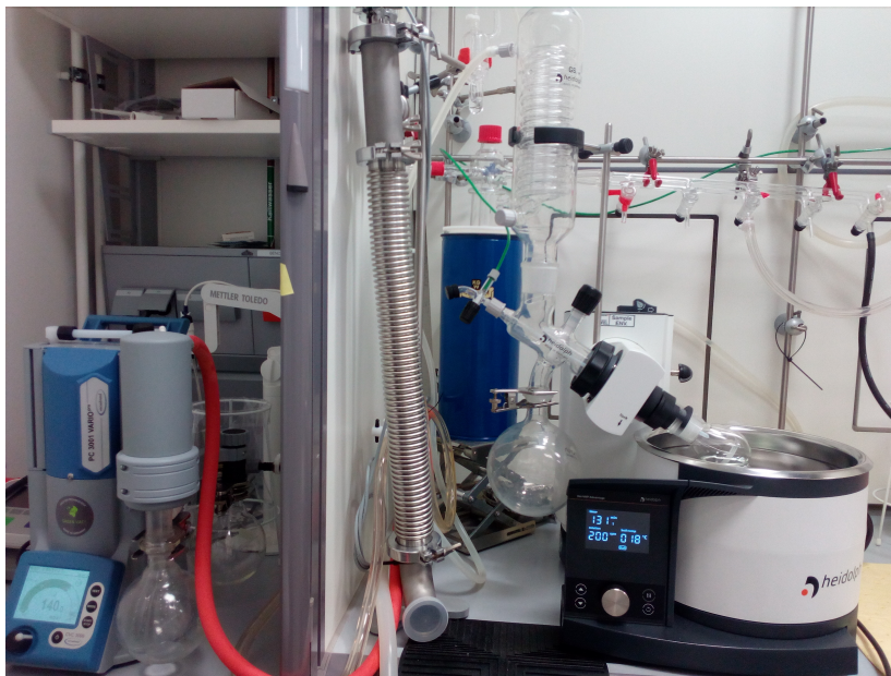
Figure 4.4: Setup of the Rotary Evaporator connected to the Schlenk line and vacuum pump. The Schlenk line provides nitrogen flow into the system and the ice cold water bath prevents oxidation of the precipitating mixture.
