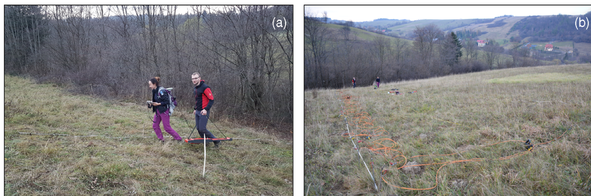
FIGURE 3 A conductivity meter EM38-MK2 (a) and the LUND electrical imaging system with SAS 4000 Terrameter (b) used in the study area [Color figure can be viewed at wileyonlinelibrary.com ]
