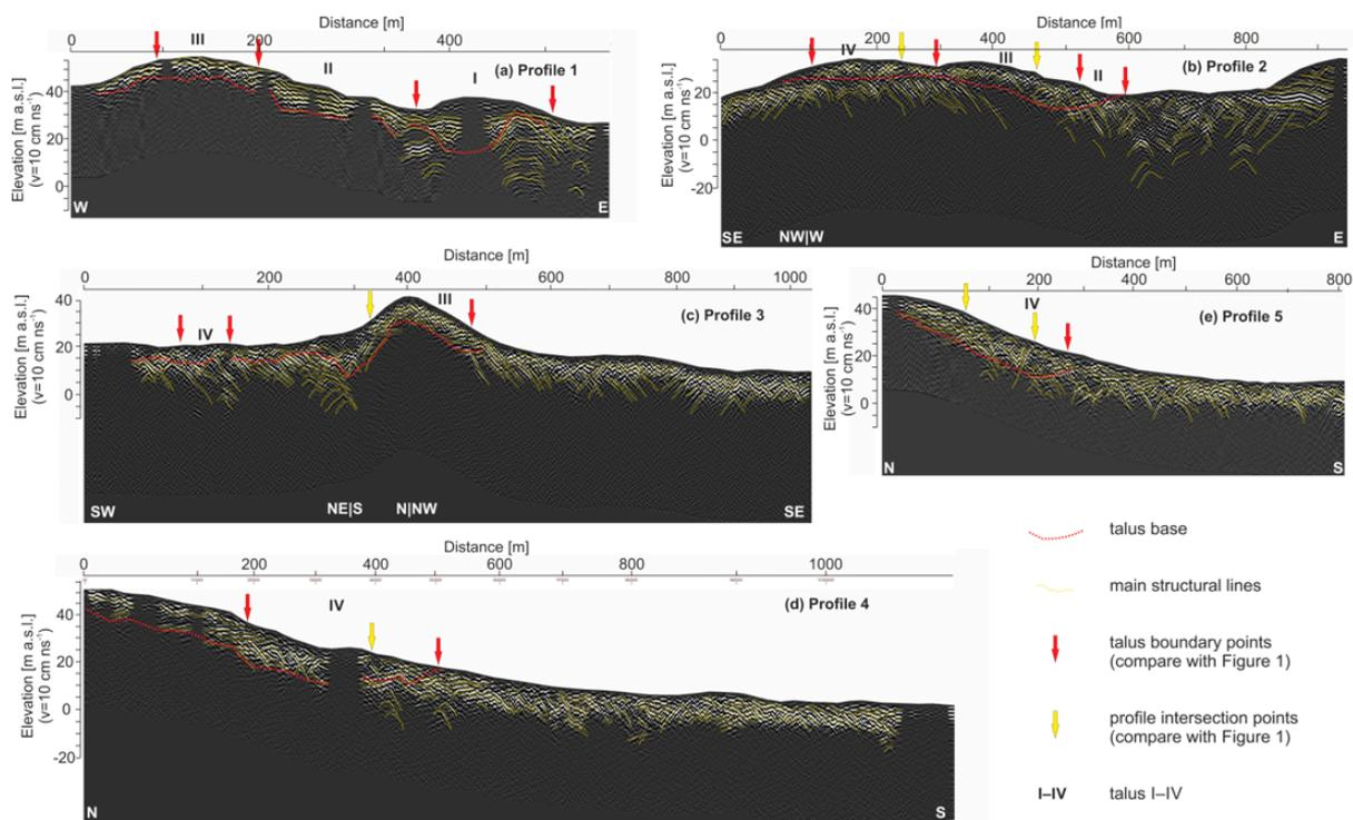
**Figure 5.** GPR profiles (30 MHz) of the talus slope on the Fugleberget mountainside. (a)–Profile 1, (b)–Profile 2, (c)–Profile 3, (d)–Profile 4, (e)–Profile 5. See Figure 1 for the location of Profiles 1–5.
