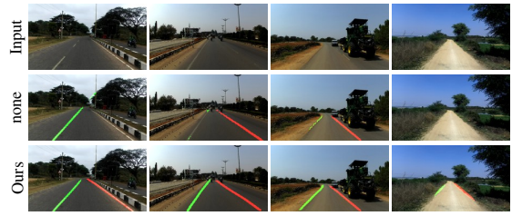
Figure 7: SCNN (Pan et al., 2017) lane detection on IDD (Varma et al., 2019). Training on generated images with degraded lanes makes existing lane detectors – such as SCNN (Pan et al., 2017) – resistant to scenes with damaged (first three columns) or no (last column) lane markings.
