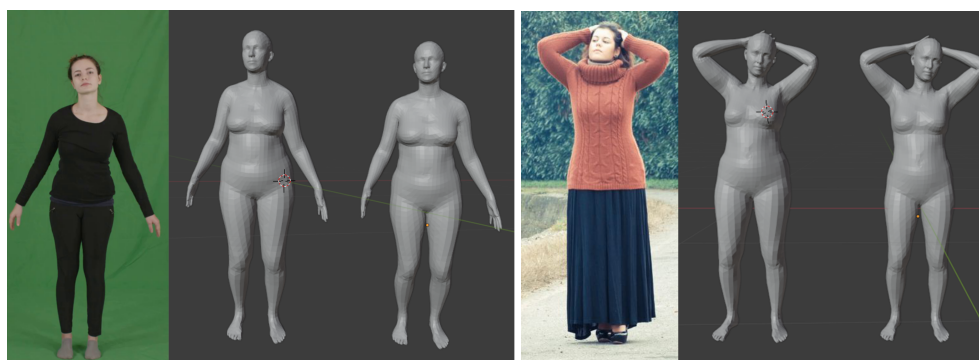
Figure 4. Qualitative examples of body reconstruction from an image of the People Snapshot (left) and an “in the wild” image (right). The two reconstructions are obtained using the HMR method (left) and our approach after Phase 2 (right).
