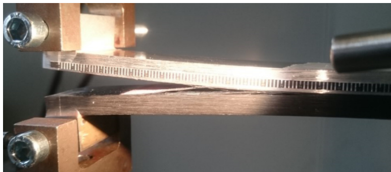
Figure 28. Detail of crack in the composite adherend (DCB_AF163_03 test) where it is evident that it converts into delamination after a certain propagation.
