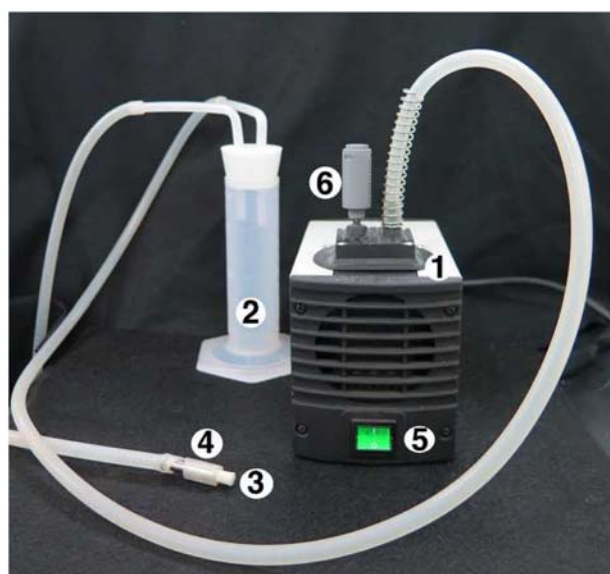
Figure 1. The micro-aspiration device: the membrane pump connected to the luer-lock brush, and the trap inserted within the suction tubing.
