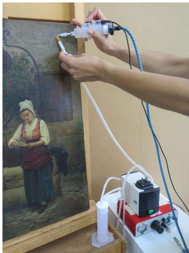
Figure 6. The use of the controlled application micro/ aspiration system on a painting in an upright position on the easel.
