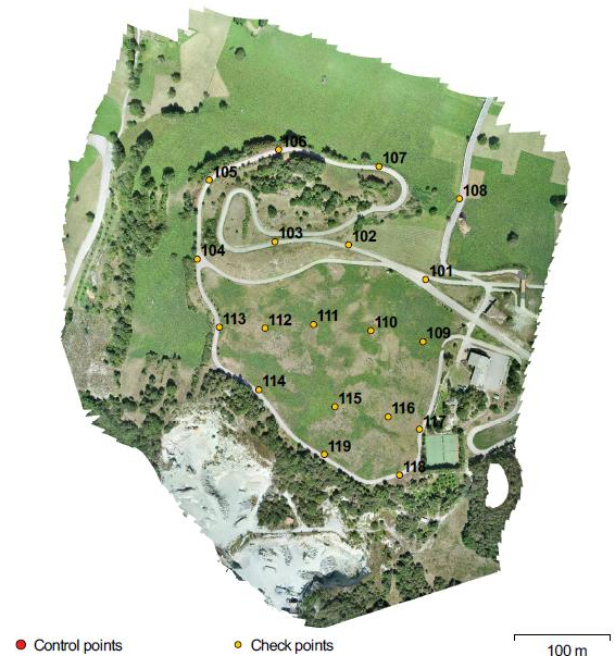
Figure 1. The survey area and the target locations. Most targets act only as check point; some is used as GCP in some tests
