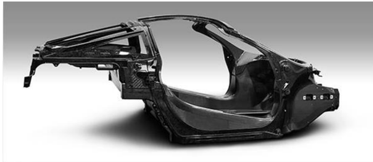
Fig. 1. Example of CF-SMC automotive chassis produced by CM, [5].
