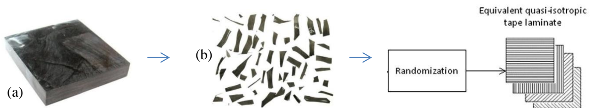
Fig. 3 (a) CF-SMC material volume; (b) the CF fiber strands of the volume after matrix elimination; (c) schematic representation of the material implementation in the model
