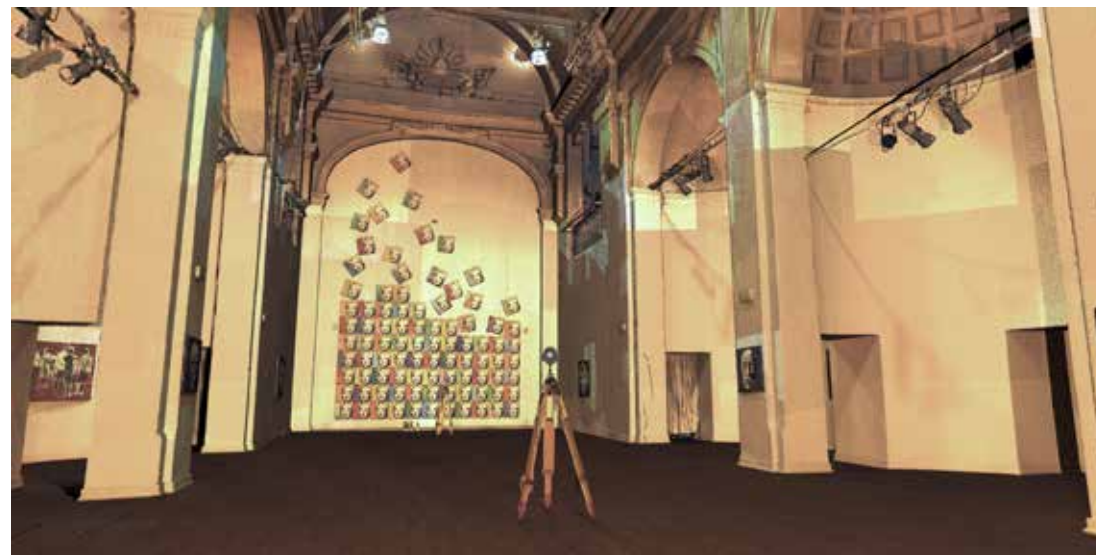
Fig. 3. Snapshot of the point clouds obtained by the laser scanner survey of the interior of the former church of Saint Ludovico, now used as an exhibition gallery for temporary exhibitions.
