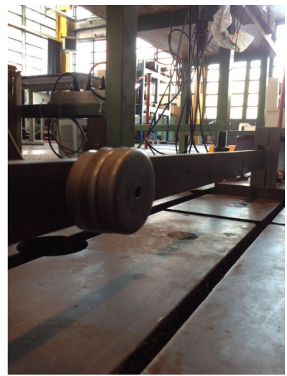
Fig. 11 Magnets added into beam
