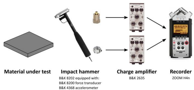
Fig. 2. Experimental setup for the apparent mass characterization of the standard skin candidates. A sample of the material under test is excited with a Brüel & Kjær 8202 impact hammer, equipped with a Brüel & Kjær 8200 force transducer and a Brüel & Kjær 4368 accelerometer. The transducers are conditioned using two Brüel & Kjær 2635 charge amplifiers. The resulting voltage signals are simultaneously acquired using a Zoom H4n recorder.
