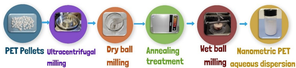
Scheme 2. Schematic representation of the production steps of label-free PET NPs.
