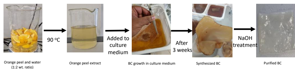
Figure 1. Schematic illustration of BC synthesis from orange peel extract.
