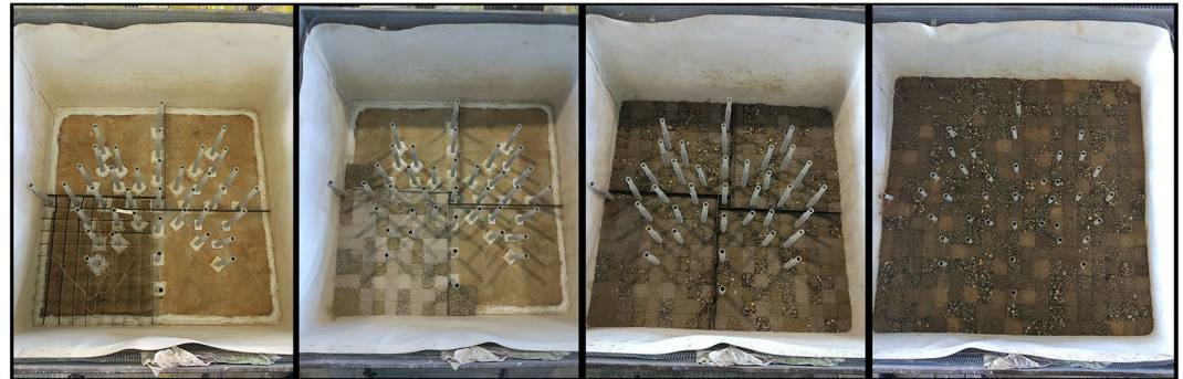
Figure 2. Illustration (from the left to the right) of the sequence leading to the layers of inclusions making up the formation.
