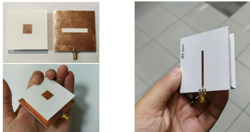
Figure 4. Top view of both the resonator element and the slotted ground plane disassembled (on top left corner ). Top frontal views of the assembled DRA (on bottom left corner ). Bottom view of the assembled DRA (on the right).
