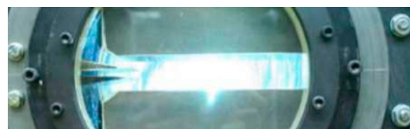
Figure 27. Example of color Schlieren out of supersonic nozzle in an air-to-air ejector (left), experimental apparatus (right). Reprinted with permission from Ref. [44] (2013).
