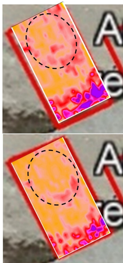
Figure 4. Depth slices in Area 2 (200 MHz). ( Upper panel ): 20 ns (110 cm). ( Lower panel ): 25 ns (138 cm).
