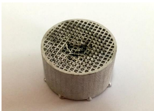
Fig. 2. Example of a defective foam sample obtained by investment casting
