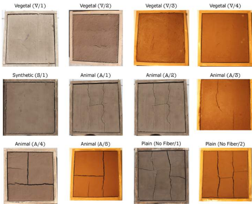
Figure 11. Dataset of samples generated from ECMs reinforced with different fiber types and a plain ECM. Samples were taken with two light sources: natural and artificial (area under analysis 500 mm × 500 mm).
