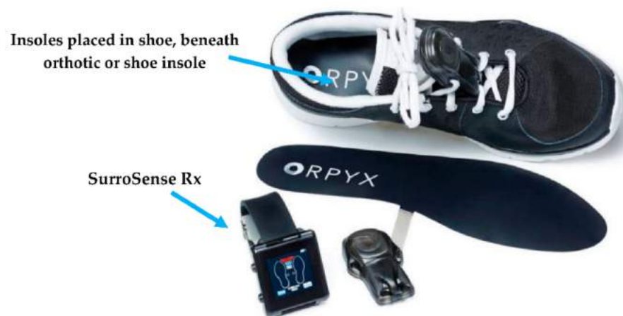
Figure 6. “SurroSense Rx” smart insole for curing plantar pressure during daily activities, Adapted from [39].
