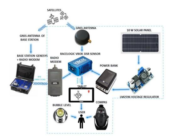
**Figure 6.** Graphical scheme of the stake-out geolocation device integrated the solar charging system (highlighted into the dashed line).
