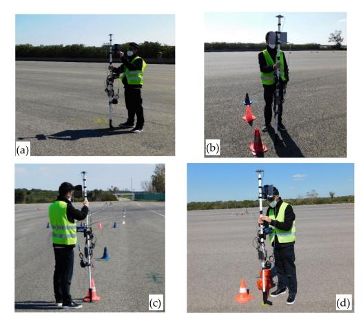
Figure 9. Use of the stake-out geolocation device to locate points with centimeter accuracy on a wide track (a-c) and record geographical coordinates of a point already marked on the ground (d).
