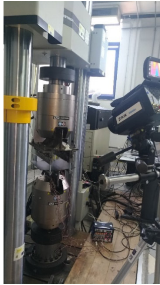
Figure 5. Experimental setup for TSA tests
