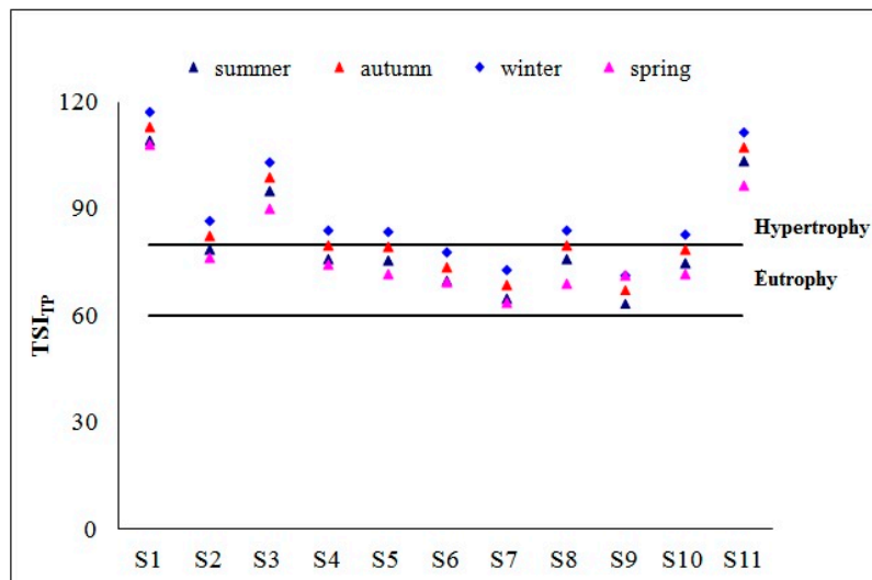
Figure 4. Seasonal trend of trophic state index ( TSI_{TP} ) determined with total phosphorus (TP). Eutrophy is recognized for TSI_{TP} values between 60–80, and hypertrophy for TSI_{TP} values above 80.
