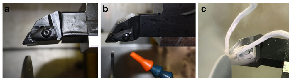
Fig. 2 Experimental setup: a dry orthogonal cutting, lubri-cooling nozzle position for b wet and c cryogenic experiments
